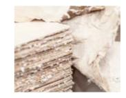
Our fibre cement consists of cement, pulp, water, plastic fibres and air. The combination of these ingredients results in a durable building material that is also lightweight compared to other cement materials. Holding the material reveals its homogeneous nature and surface quality. Its appearance highlights the unique character and natural texture.
